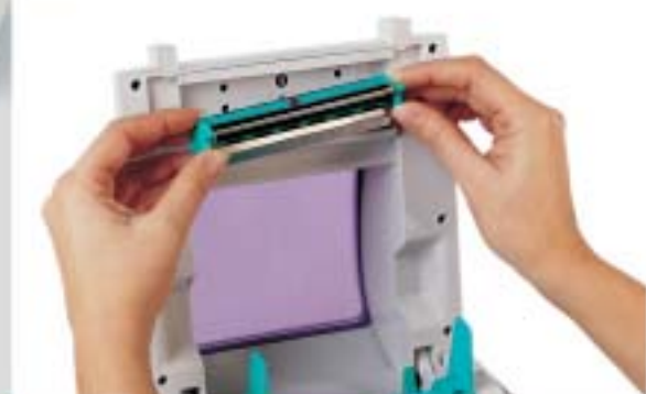
▼ Tool-less printhead replacement
